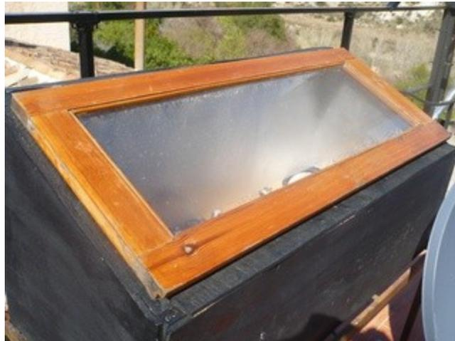
**Image 3.** A solar oven at Sunseed, used for pre-heating water to high temperatures.
