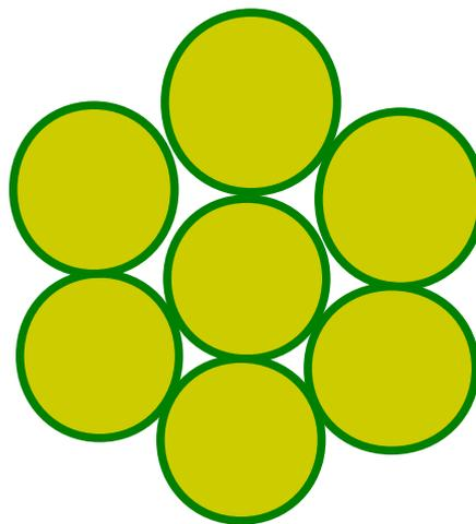
**Figure 1.** An illustrated cross-section of a caña column.
