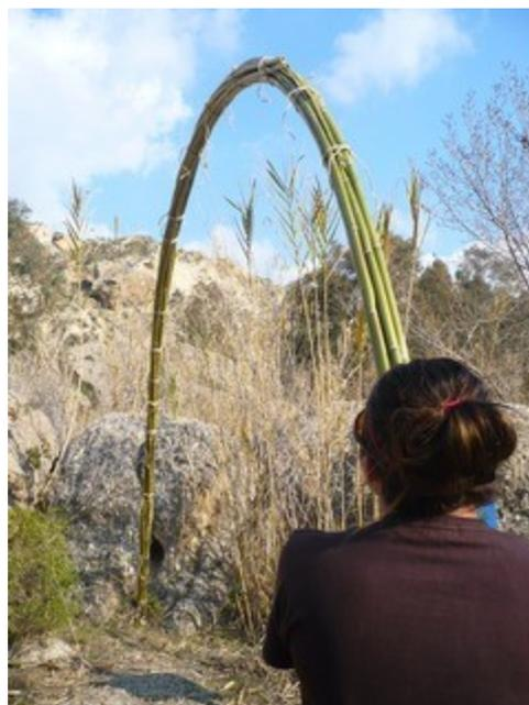
**Image 8.** Flex-testing a super-column upon assembly.
